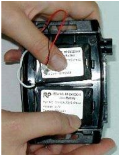
Figure 3: Battery Arrangement in the Unit Enclosure
